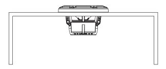
TCX models are specifically engineered for enclosed operation. This makes them ideal for wakeboard tower systems or other small enclosure applications.
